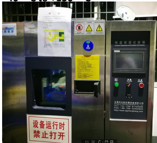
Temperature ageing testing oven -40° C to +150° C
